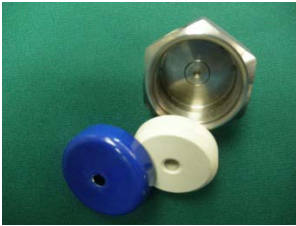
Portion of steam trap showing new ceramic insert.
