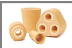
A tundish nozzle for manufacturing steel, developed by Zircoa, Solon, OH, has a fine-grained zirconia liner inside a more conventional coarse-grained nozzle. The insert has higher density and strength, and lower porosity than the surrounding material. This improves dimensional stability and resistance to erosion and corrosion.
