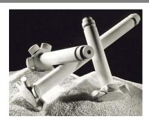
This composite-ceramic degasser removes hydrogen gas from molten aluminum. A combination of freeze molding and injection molding lets Blasch Precision Ceramics, Albany, NY, make a permeable ceramic from a silicon carbide/alumina composite. The process generates <5µm pores in the degasser head but a stronger, denser shaft.
