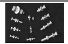
Injection-molded ceramic fasteners from Ceramco, Center Conway, NH, come in handy for non-stress applications in electrical equipment, replacing fasteners made of plastic. They are electrically insulating and work well in corrosive or high-temperature environments such as metal plating and industrial kilns.
