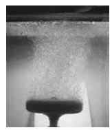
Porous ceramic replaces plastic, sintered metal, and exotic alloys in gas diffusers for corrosive, abrasive, and high-temperature applications. The Solidome™ gas diffuser made by Refractron Technologies, Newark, NY, is used in the aeration and oxidation of various liquids. A ceramicmembrane coating process produces diffusers with pore sizes from 0.1 to 30 µm.
